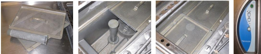
1. Ensure plug and filter plates in position
